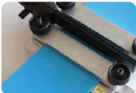
Welding narrow flat belts with Pliers P-200
