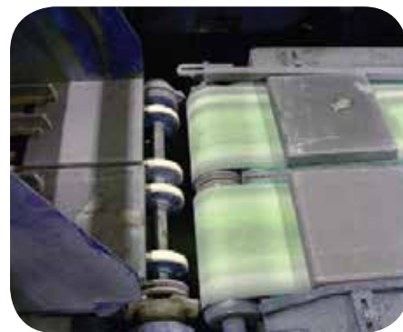
FK - 3 Brick pre - oven conveying
