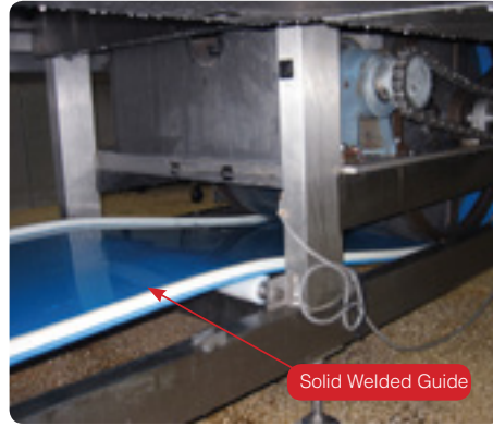
2. Two parallel guides on, or close to the belt edges on the underside of the belt used on wider belts; common in vegetable processing.
